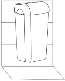
1. fix the plate to the wall with screws-kit
