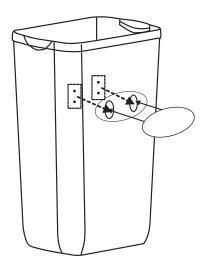
2. fix the plate to the bin with the rectangular plaques
